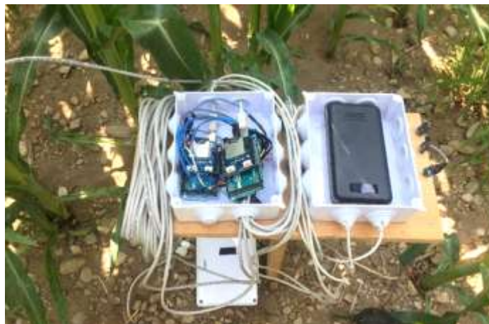
Soil moisture/air and air temperature measurement sensors based on Arduino Mega 2560 card
