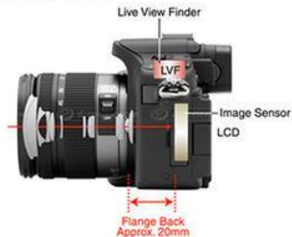
Mirror-Less Structure (DMC-G1)
