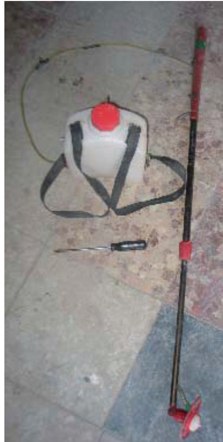
Figure 3. Battery-operated sprayer with centrifugal spray tip.
