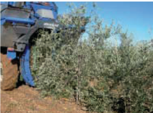
Figure 31. Over-the-top harvester in super-intensive orchard.
