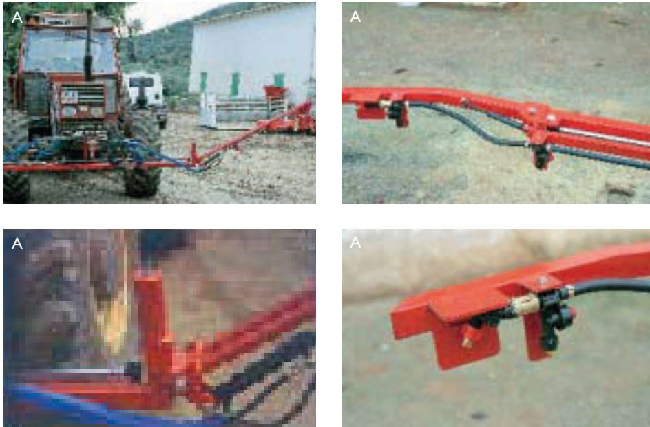
Figure 6. (A) Close-ups of boom sections and end spray tip arrangement. (B) Adaptation to changes in slope.
