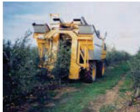
Figure 25. Shaker featuring larger shaker cage.
