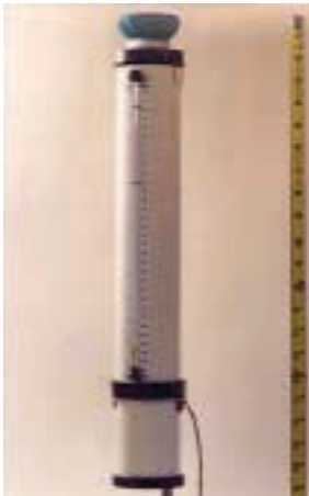
Figure 2. Atmometer (from Altenhofen, 1985)
